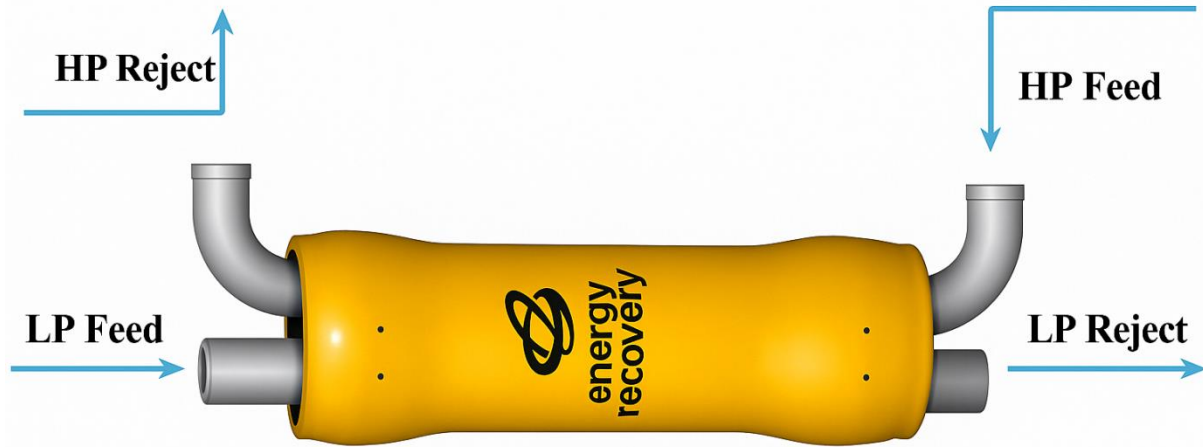
Fig.6. Energy recovery device
